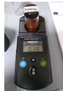
Figura 13. POCKET Colorimeter II
